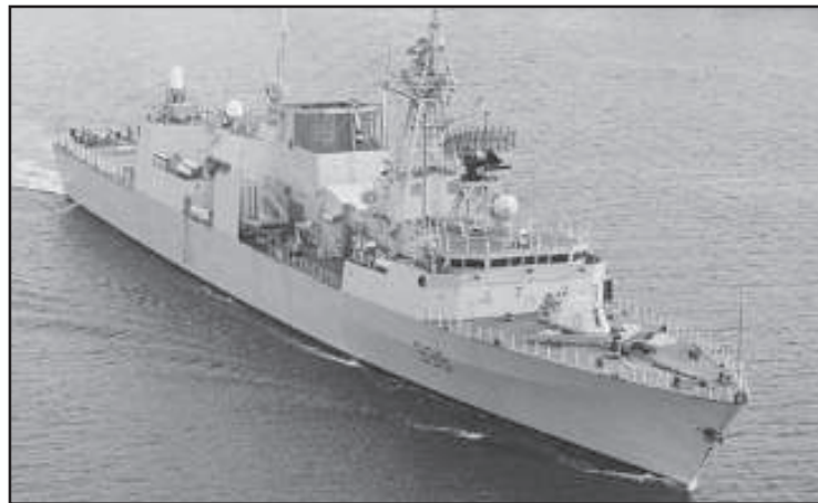
The armament carried by the HMCS Charlottetown includes 24 Honeywell Mk 46 torpedoes, 16 surface-to-air missiles, 8 anti-ship harpoon missiles, six .50 caliber machine guns, a 57 mm Bofors Mk2 gun, and a Phalanx close-in anti-ship weapons system manufactured by General Dynamics.
